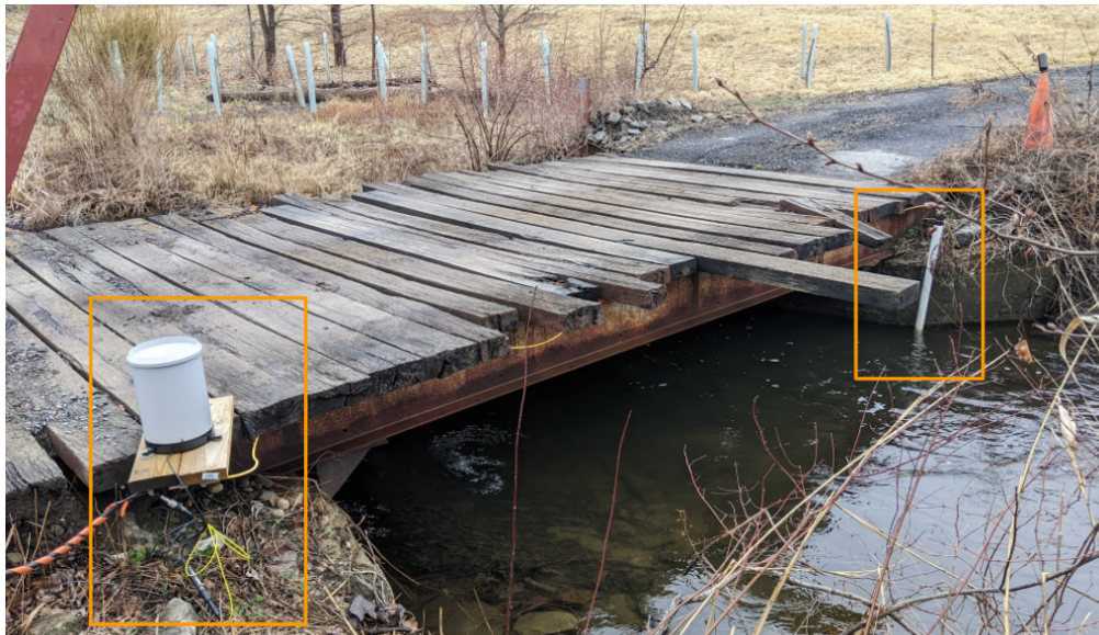
Figure 2: The equipment installation site during the March 25 site visit, with the tipping bucket (left) and the LevelVent Logger (right).
