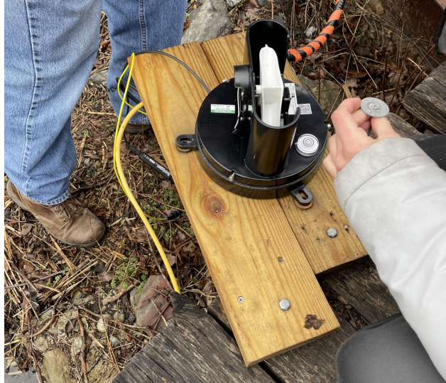
Figure 4: The interior mechanism of the tipping bucket during assembly
