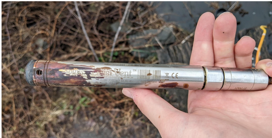
Figure 3: The Solinst LevelVent Logger taken out of the stream during the March 25 site visit.
